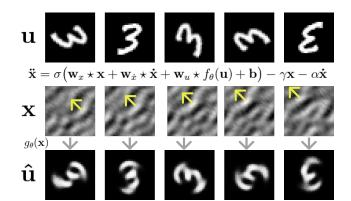
Figure 1: Overview of the Neural Wave Machine. The input sequence **u** is encoded with  $f_{\theta}$  to act as a driving term in the hidden state **x** which is modeled temporally ( $\ddot{\mathbf{x}}$ ) as a network of locally coupled oscillators. The network is then trained to reconstruct the input sequence:  $\hat{\mathbf{u}} = g_{\theta}(\mathbf{x})$ . The yellow arrows track a traveling wavefront over time.
